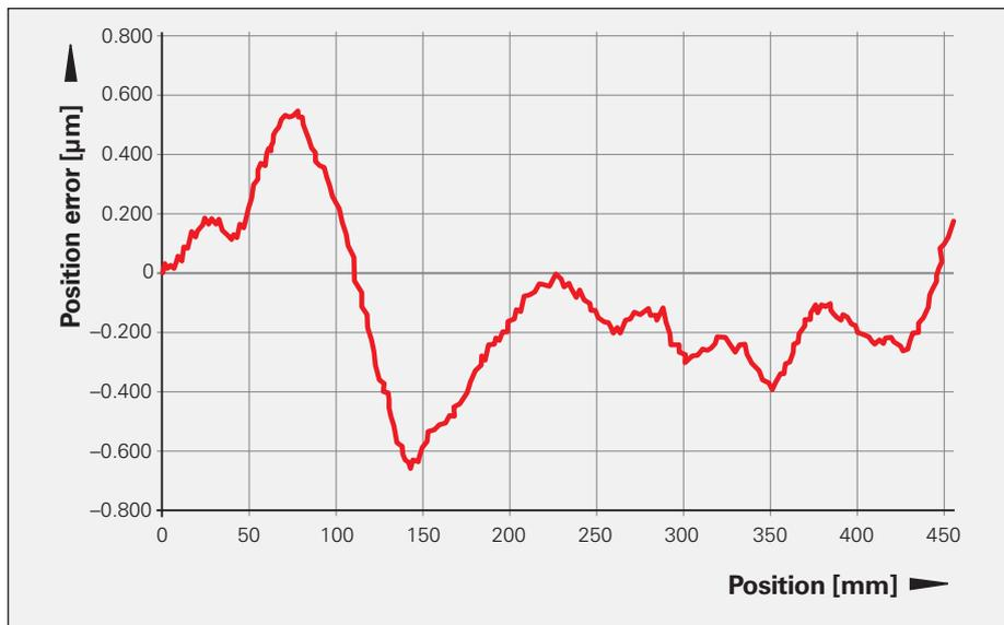
Figure 1: Typical position error over measuring length
