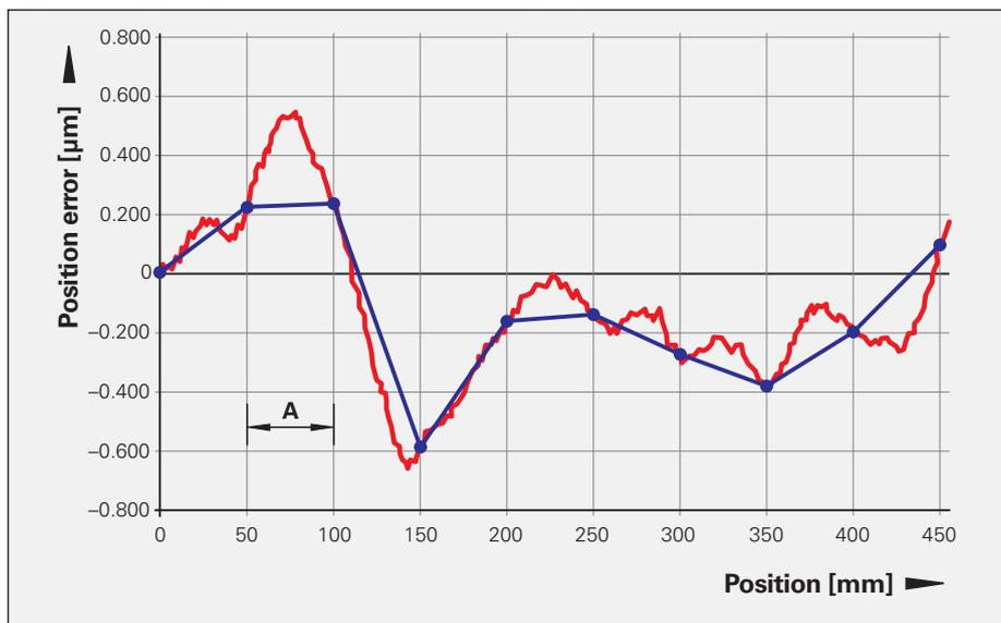
Figure 2: Compensation points for multipoint linear error compensation
